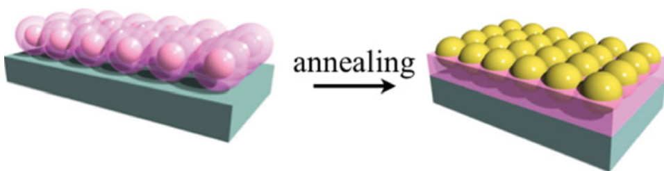
Figure 1. Concept images of OPV inner structure using hybridized nanocrystals before and after annealing.
